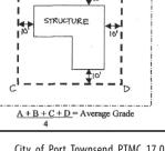
City of Port Townsend PTMC 17.08.020 "Building height" means the vertical distance from the average natural (preexisting) grade to the highest point of the coping of a flat roof or the deck line of a mansard roof or the average height of the highest gable of a pitched or hipped roof.
